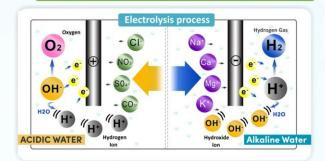
Alkaline water electrolysis is used to split water into the gases hydrogen and oxygen using electric energy. The tap water moves through several electrode plates , separating into acidic and alkaline parts. It is split into OH- (hydroxid ions) and H+ (hydrogen ions). All this takes place through natural process
